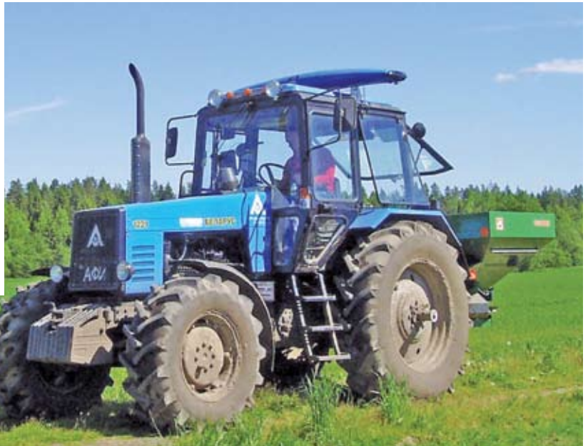
MTЗ 1221 + Amazone ZA-M + N-sensor + GPS AgGPS132
